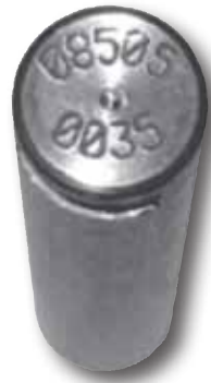
For example, this roll was assembled on the 85th day of 2005 and it was the 35th roll assembled that day.
