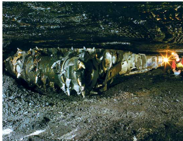
A CM210 at work in an 860 mm (34 in) seam
