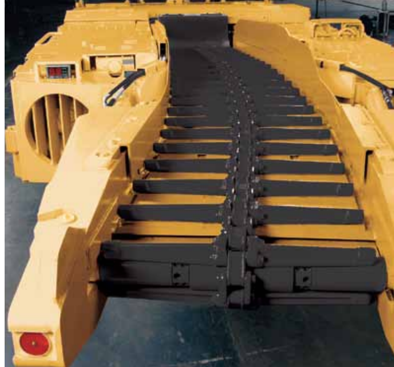
Discharge boom with automatic chain tensioner
